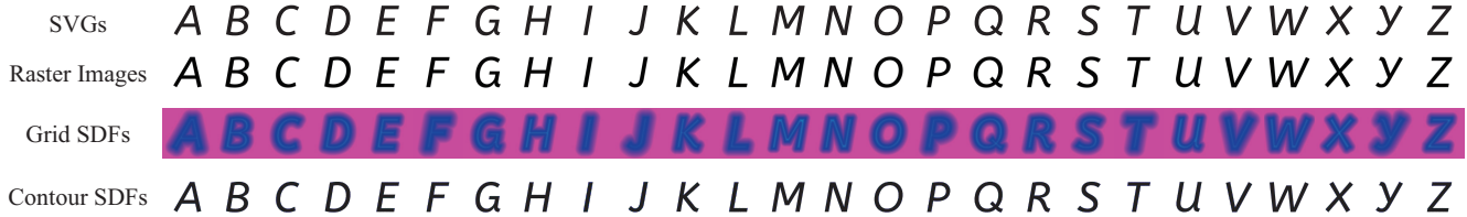
Figure 5. Examples of vector glyphs, glyph images, grid SDFs and contour SDFs. For better visualization of grid SDFs, we map the positive value of distance functions to the red channel of RGB images and map the negative value to the green channel. To visualize the contour SDFs, we add all the contour sampling points into the original SVG files. Please zoom in for better inspection.
